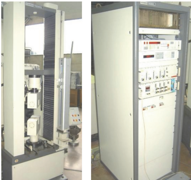
Figure 3 Electromechanical testing machine SCHENCK TREBEL RM100
