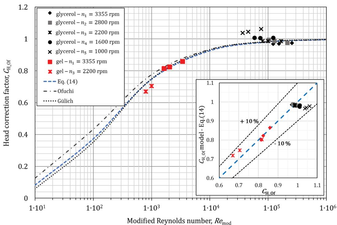
Fig. 5 – Head correction factors versus modified Reynolds number by Ofuchi method at three normalised specific speed values with Wilo-Helix-EXCEL 1602-1/16/E/KS pump.
