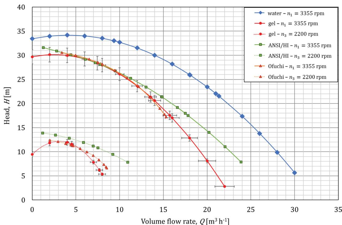
Fig. 7 – Measured (red curves ● with  $\pm 5\%$  error) and predicted performance curves with gel at different rotational speeds with measured baseline curve with water as reference (thick blue with  $\diamond$ ).
