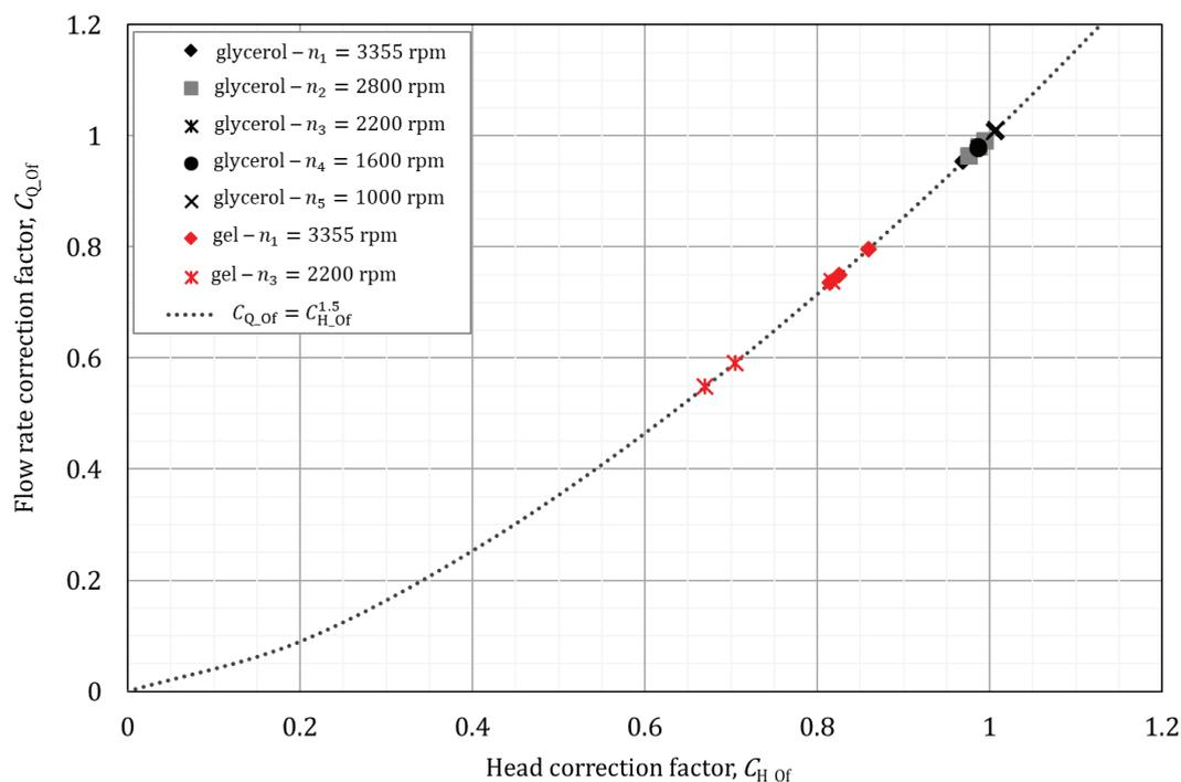
Fig. 4 – Flow rate correction factors versus head correction factors by Ofuchi method at three normalised specific speed values with Wilo-Helix-EXCEL 1602-1/16/E/KS pump
