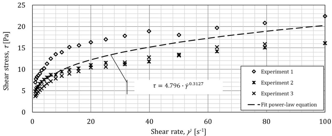
Fig. 1 – Measured and fit rheology curves of the gel
