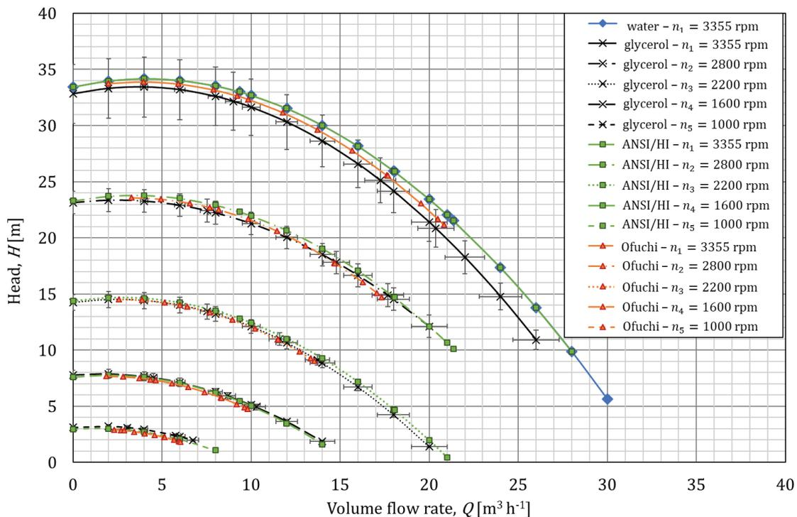
Fig. 6 – Measured (black curves with  $\pm 5\%$  error) and predicted performance curves with glycerol at different rotational speeds with measured baseline curve with water as reference (thick blue with  $\diamond$ ). Green  $\square$ : predicted with ANSI/HI method, orange  $\Delta$ : predicted with Ofuchi method.
