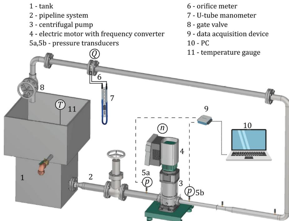
Fig. 2 – Experimental setup
