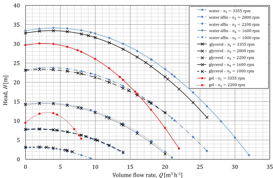
Fig. 3 – Performance curves of the pump: measured at nominal speed and calculated with affinity-law for other rotational speeds with water (blue  $\diamond$ ); measured with glycerol (black  $\times$ ) at five rotational speeds, and with gel (red  $\bullet$ ) at two rotational speeds
