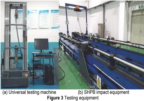
To prepare the SHPB impact test, the sample needed to be placed at the designated position, and the axial stress of 0.1 MPa was applied by the axial loading device to ensure the close contact between the specimen and the testing apparatus without falling off. The schematic diagram of impact devices is shown in Fig. 4.
