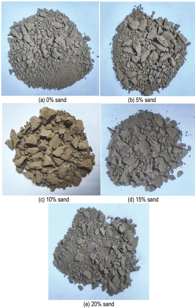
Figure 12 Failure patterns of specimens under various sand content (impact load 0.3 MPa)
