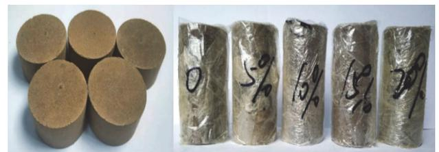
(a) SHPB specimens (b) Compressive strength specimens
