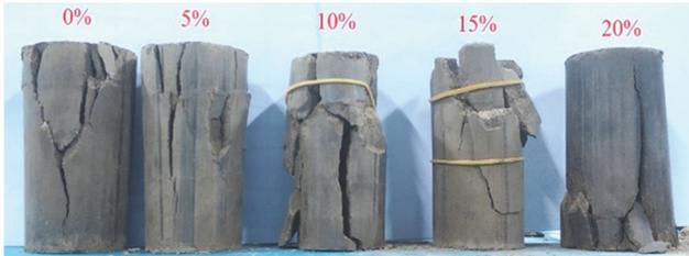
Figure 6 Failure mode of unconfined compressive strength
