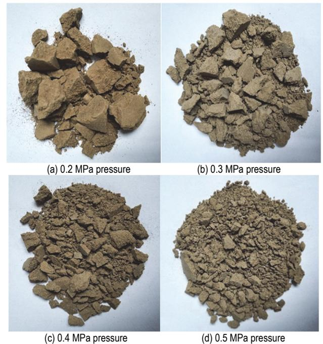
Figure 11 Failure patterns of specimens under impact loads (sand content 10%)
