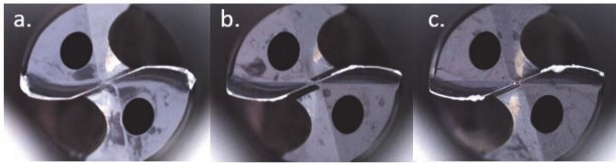
Figure 10 Tool wear at the end of the test with a. 200 m/min; b. 165 m/min; c. 110 m/min
