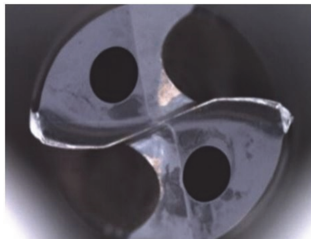
Figure 5 Wear on clearance face
