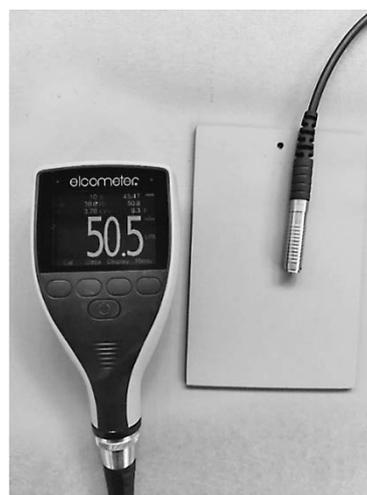
**Figure 3** Measuring of the dry film thickness formed by the primer with the dry film thickness of 45  $\mu\text{m}$
