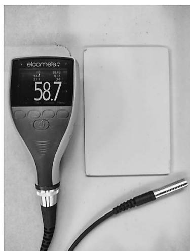
**Figure 2** Measuring of the dry film thickness formed by the primer with the dry film thickness of 60  $\mu\text{m}$
