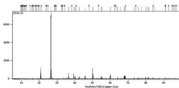
**Figure 2** X-ray spectrum in the powdered form of the CHM sample (phase peaks are shown, sample No. 3). Peaks of quartz sand
