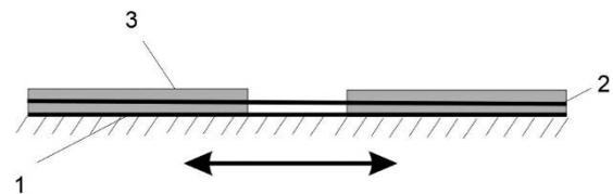
**Figure 2** Advanced sensor design without an optical fiber loop (sensor): 1 – side face of the beam, 2 – optical fiber, 3 – optical fiber loop (sensor), 4 – layer of epoxy glue
