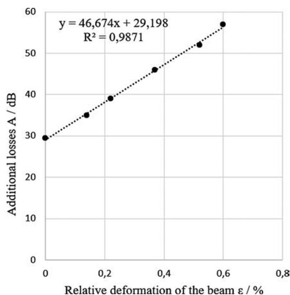
**Figure 4** Graph of the additional losses of a light wave growth with increasing mechanical stresses of the beam
