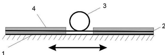
**Figure 1** Sensor design having an optical fiber loop (sensor): 1 – side face of the beam, 2 – optical fiber, 3 – optical fiber loop (sensor), 4 – layer of epoxy glue [1]
