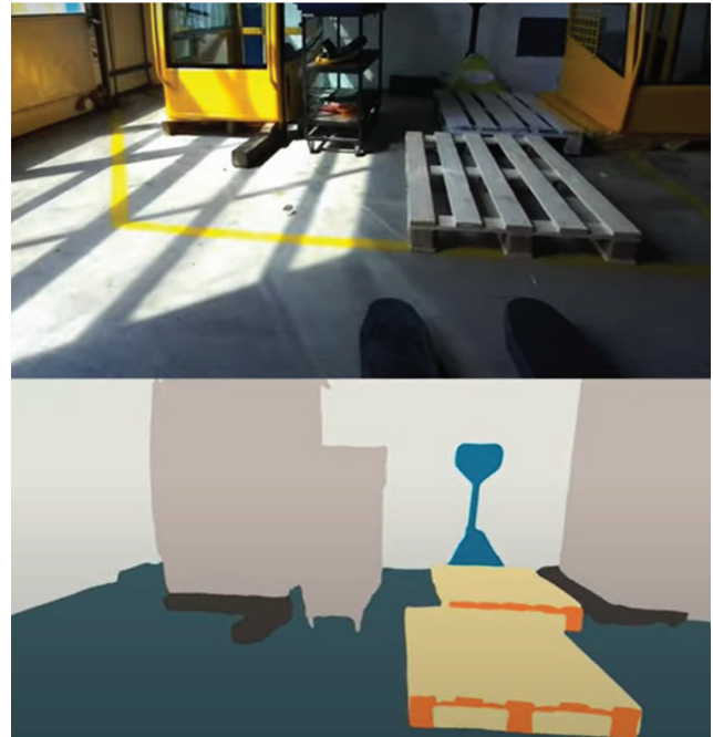
Figure 3. Visual perception for a pallet pickup
