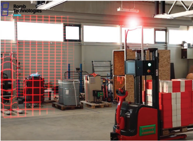
Figure 2. Natural localization (artistic depiction of laser scan). A laser on the top of the AGV measures distances from the objects surrounding the AGV, thus providing data for an algorithm that an artificial grid of occupied and free spaces around the vehicle
