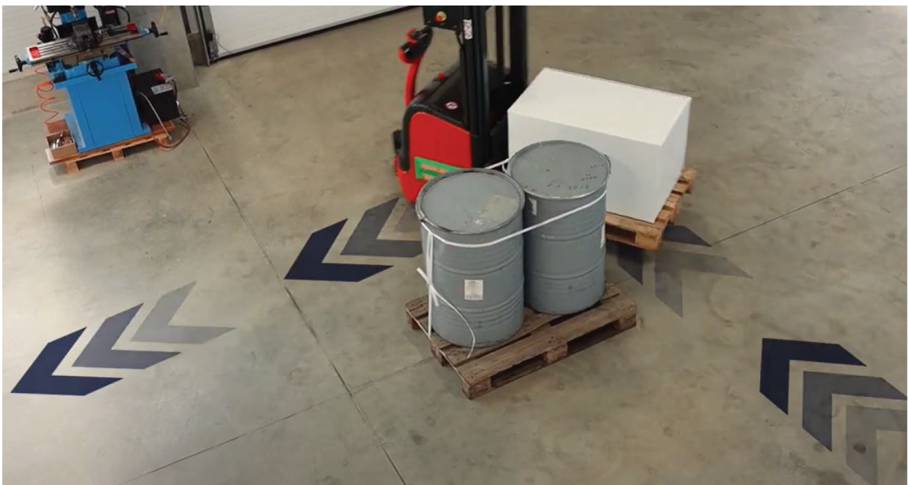
Figure 4. An AGV passing next to an obstacle by using MPC-based path following
