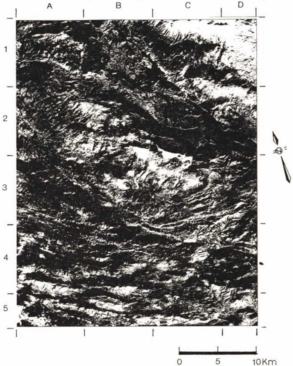
Figure 3. Combined edge enhanced image using both filters A + W and B + W with a histogram equalisation contrast stretch, enhancing both NW-SE and NE-SW edges.
