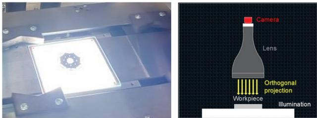
Figure 5 Illumination and sketch of the acquisition system
