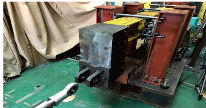
Figure 10 Actuator and Experimental setup connection part
