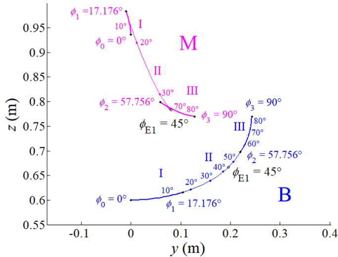
Fig. 7 Metacentric M-curve for rectangular cross section in the first quadrant
