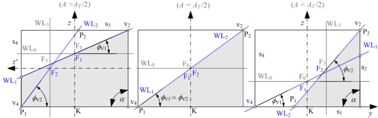
Fig. 4 Deck immersion/bottom emersion immersion shapes for rectangle
