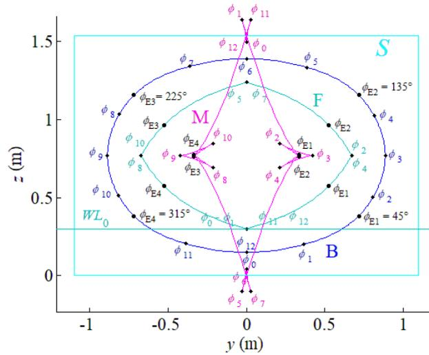
Fig. 10 Hydrostatic properties for rectangular cross section pontoon, case  $A/A_T < 1/2$
