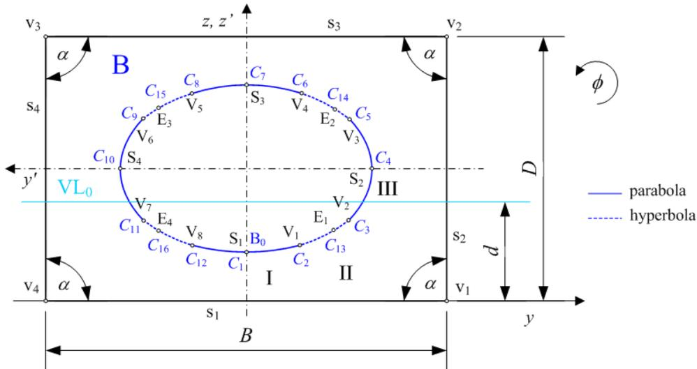
**Fig. 1** Rectangular cross shape centre of buoyancy segments with cusp discontinuities
