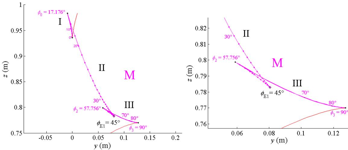
Fig. 8 Metacentric M-curve with zoom of extreme cusp discontinuity for hyperbola
