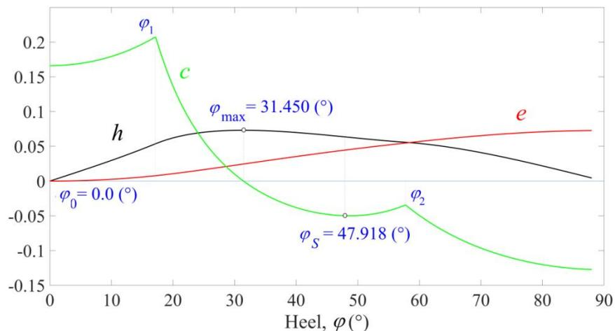
**Fig. 12** Elementary transversal stability functions for draught  $d = 1.2$  (m)
