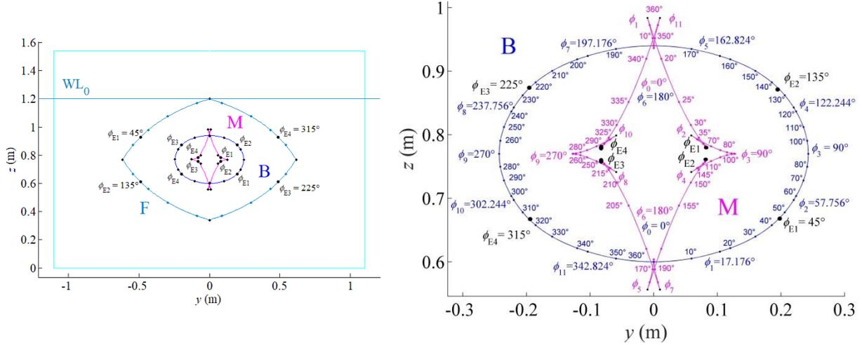
Fig. 9 Hydrostatic properties for rectangular cross section pontoon, case  $A/A_T > 1/2$
