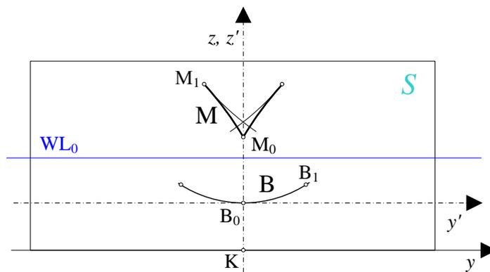
**Fig. 2** Symmetric semi-cubical parabola M curve with butterfly type discontinuity
