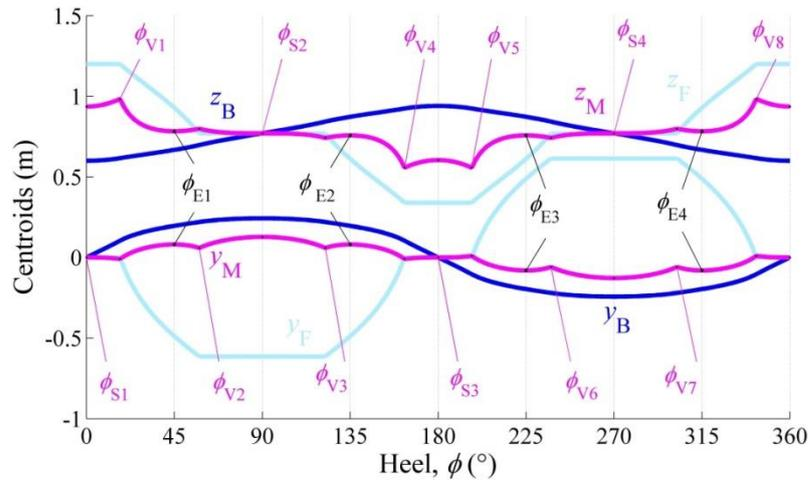
**Fig. 5** Hydrostatic particulars centres components for heel angles  $\phi$  for rectangle
