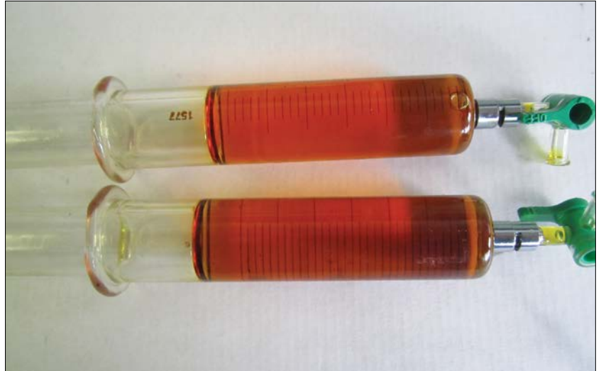
Figure 5. A bubble enters the syringe during air transportation
