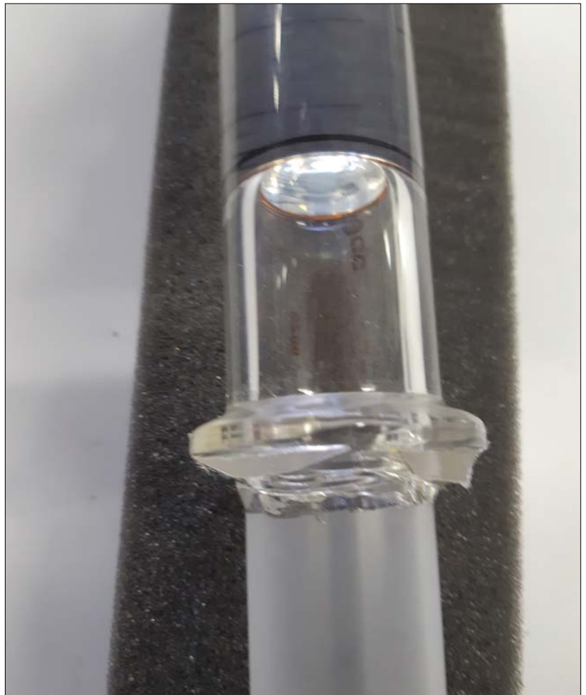
Figure 6. A sealed syringe prepared for air transportation - the sealing between the piston and body prevents leakages
