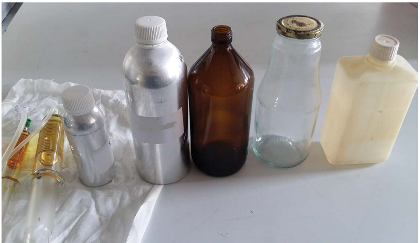
Figure 7. Acceptable vessels for DGA and oil tests
