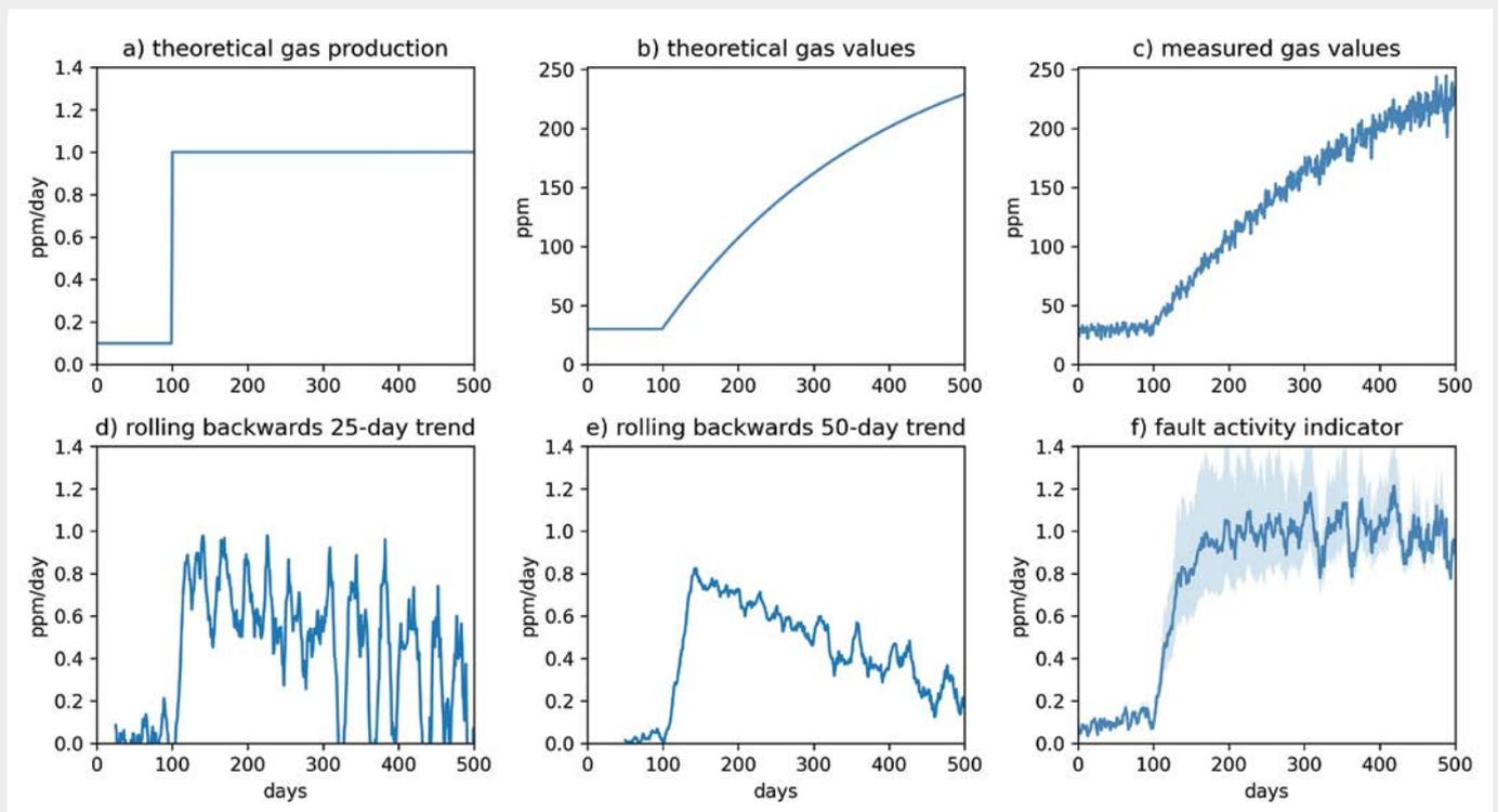
Figure 3. Implementation of different trending algorithms
