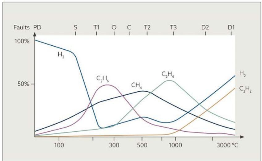
Figure 2. Gas formation pattern as a function of temperature [3]
