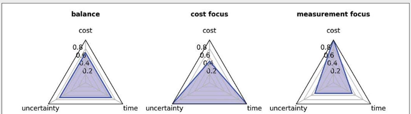
Figure 5. Relationship between costs, measurement uncertainty and measurement time for analyzer systems
