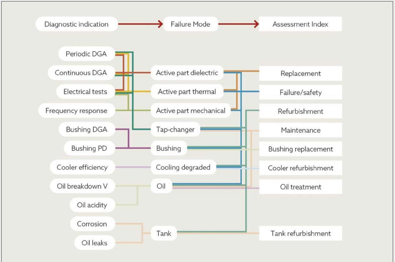
Figure 1. Relationships between diagnostic methods, failure modes, and assessment indices [1]
