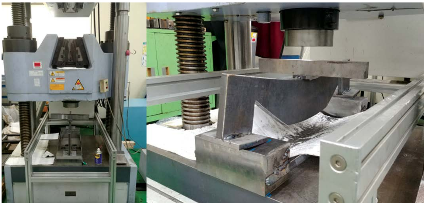
Figure 8. Stiffener flexibility check
