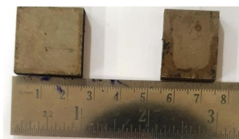
Figure 1. SS-304 substrates obtained after WEDM cutting
