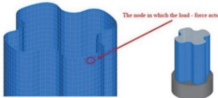
Figure 6 Mesh view of the machining workpiece
