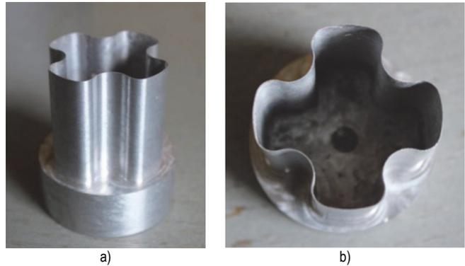
Figure 13 Photographic representation of the manufactured workpiece (pocket) and the final process of decomposition of the mixture of natrium silicate and fireclay flour with water after the completion of the machining process
