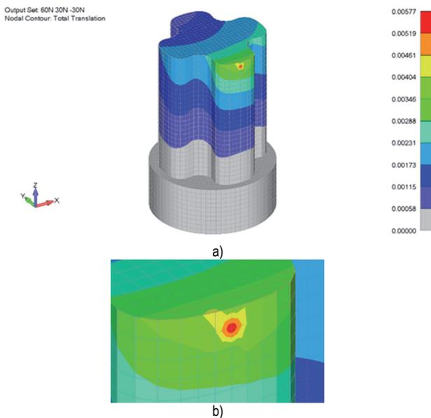
Figure 8 a) Total displacements; b) Magnified detail of the workpiece on which the tool load acts during machining
