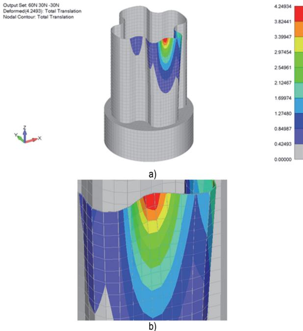
Figure 11 Displacement field in the case where the pocket is not filled with a mixture of natrium silicate and fireclay flour
