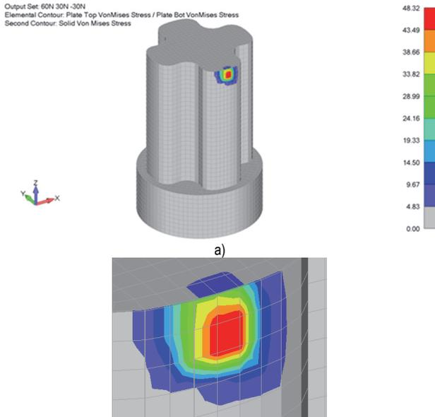
Figure 7 a) Stress field-Whole model; b) Magnified detail of the workpiece on which the tool load acts during machining
