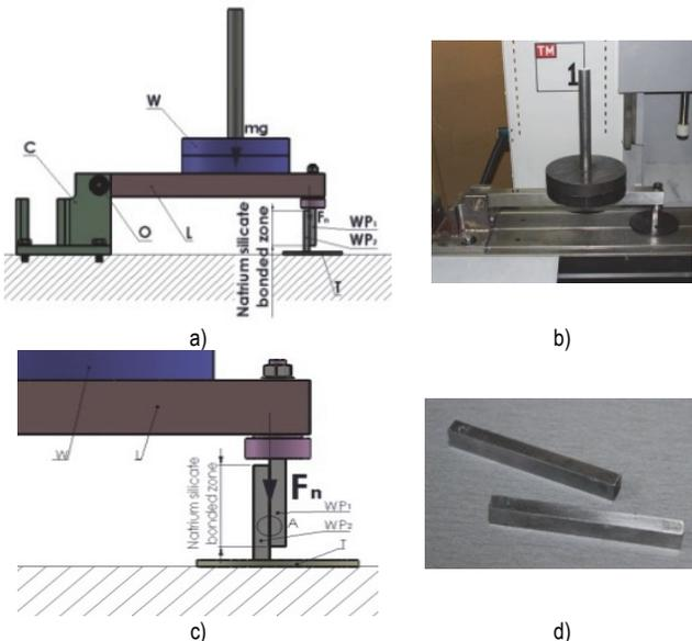
**Figure 1** CAD model of purpose-built test device (a); photographic representation of the device (b); CAD detail of the bond breaking zone under the action of shear stress (c); photographic representation of the samples after breaking the bond (d)
