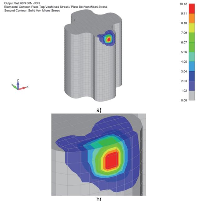
Figure 9 a) Stress field - Whole model; b) Enlarged detail of the workpiece where the tool load is transferred through the thin wall
