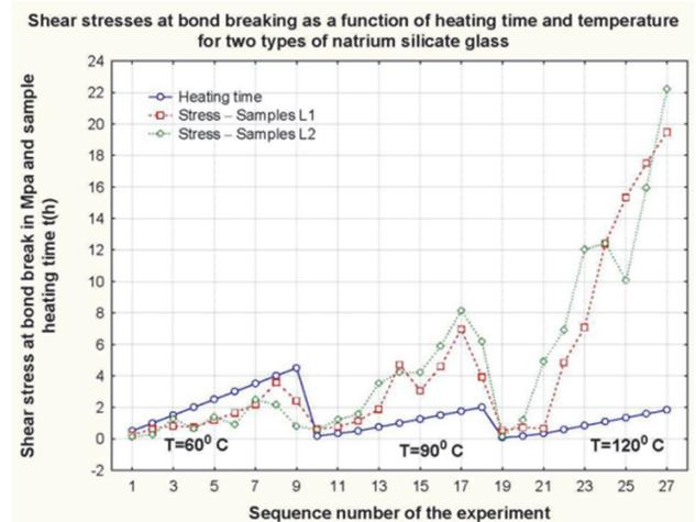
**Figure 3** Bearing capacity of the joint from the aspect of shear stress
