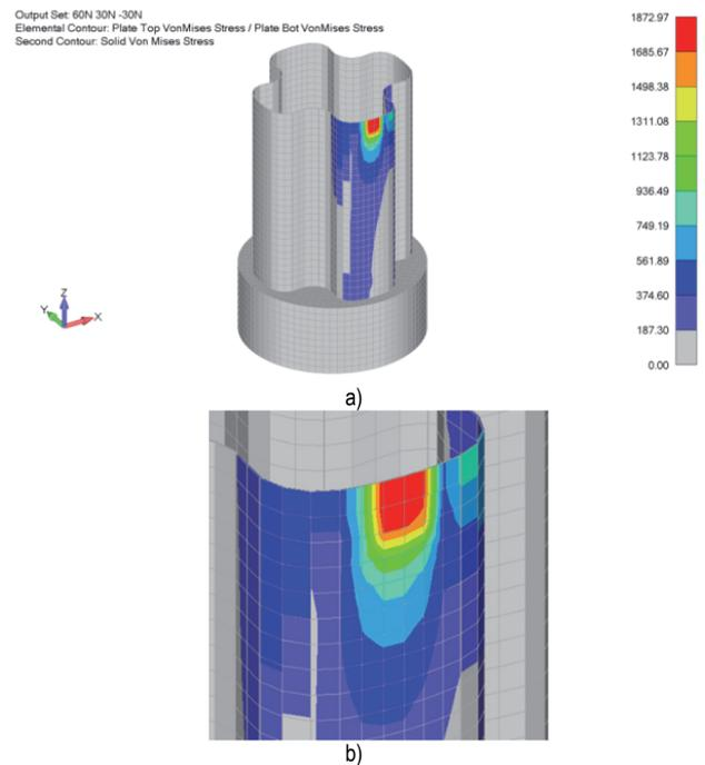
Figure 10 Stress field in the case where the pocket is not filled with a mixture of natrium silicate and fireclay flour
