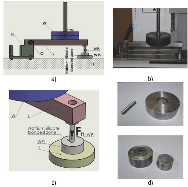
**Figure 2** CAD model of purpose-built testing device (a); photographic representation of the device (b); CAD detail of the bond breaking zone under the action of tensile stress (c); photographic representation of the samples after breaking the bond (d)
