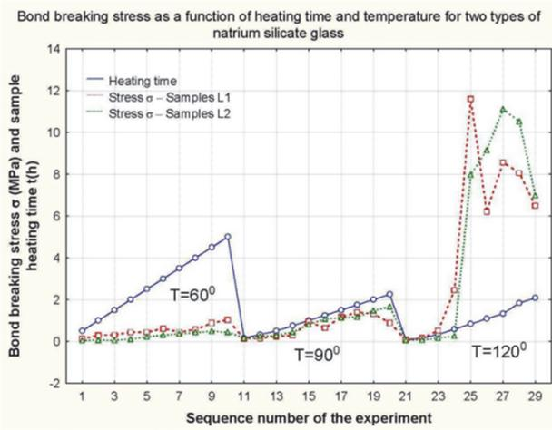
Figure 4 Bearing capacity of the joint from the aspect of tensile stress
