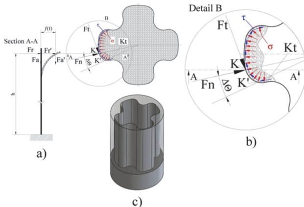
Figure 5 Stress and deformation state of the thin-wall workpiece of the closed contour during the machining. Cross section A-A of figure b (a); Magnified view of the workpiece from above (b); Isometric view of the workpiece with transparently marked edges of the workpiece before machining (c)
