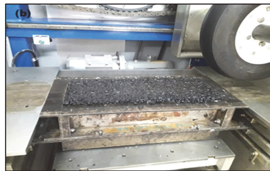
Figure 5 Preparation of the mold for fatigue test
