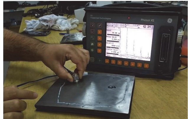
Figure 6 Welded joint testing with ultrasound
