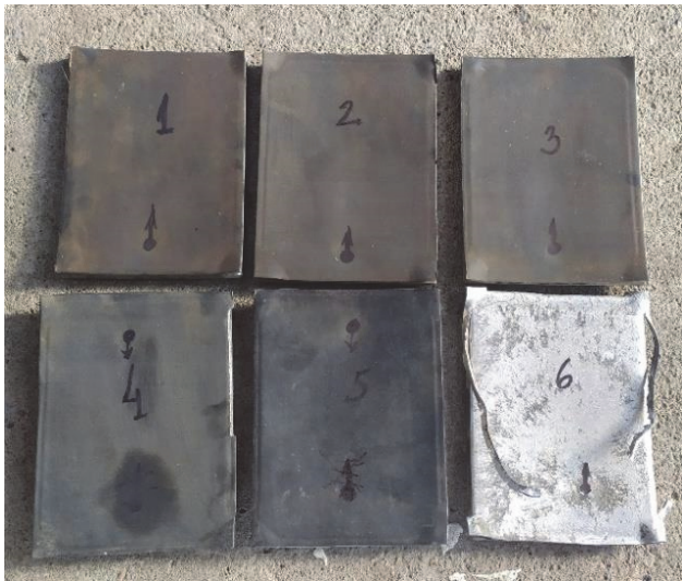
Figure 5 Plates obtained by explosive welding
