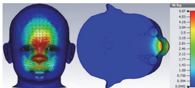
Figure 6 Distribution of \text{SAR}_{1\text{g}} / \text{W}/\text{kg} for the child head model's distance of 3 cm from the phone
