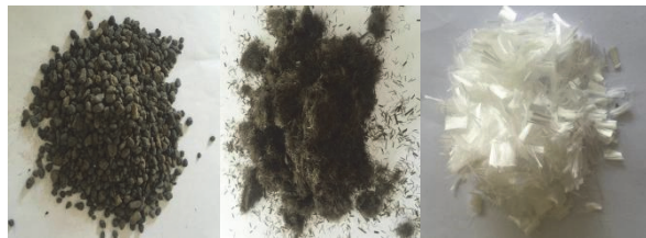
(a) shale ceramsite (b) basalt fiber (c) polypropylene fiber Figure 1 Raw materials of HFSC
