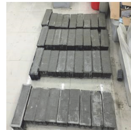
Figure 2 Concrete sample for mechanical property test
