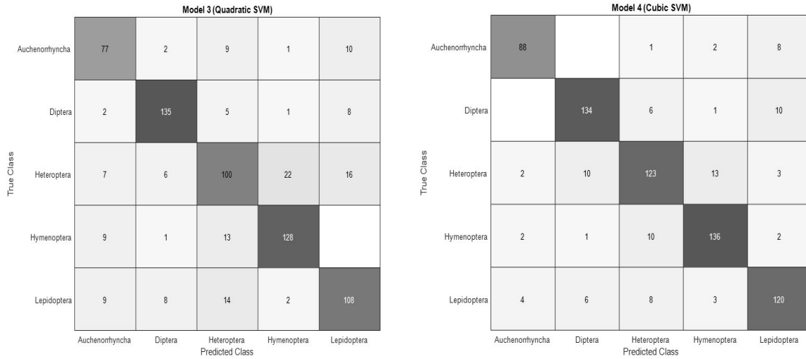
Figure 5. (left) Output-based confusion matrix after applying quadratic SVM technique on the insect image dataset, (right) output-based confusion matrix after applying cubic SVM technique on the insect image dataset.
