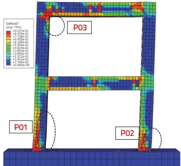
Figure 7. Damaged double-storey portal
