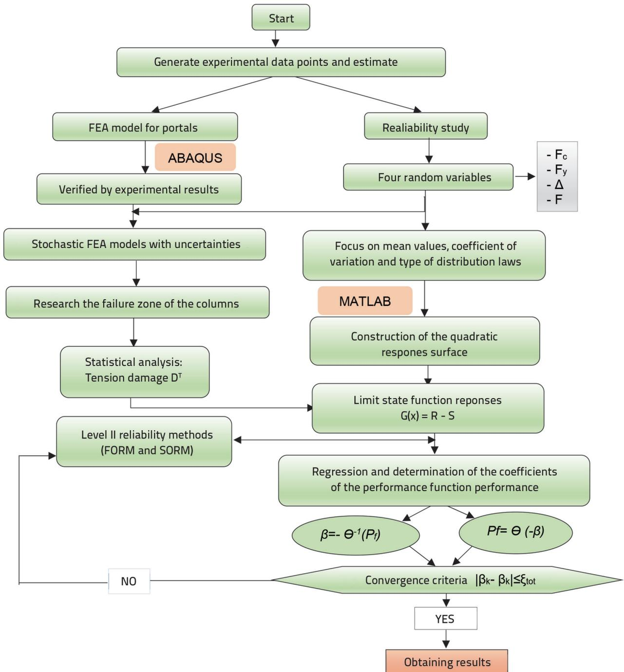
Figure 3. Flow chart of a mechanical-reliability coupling (ABAQUS-MATLAB)
