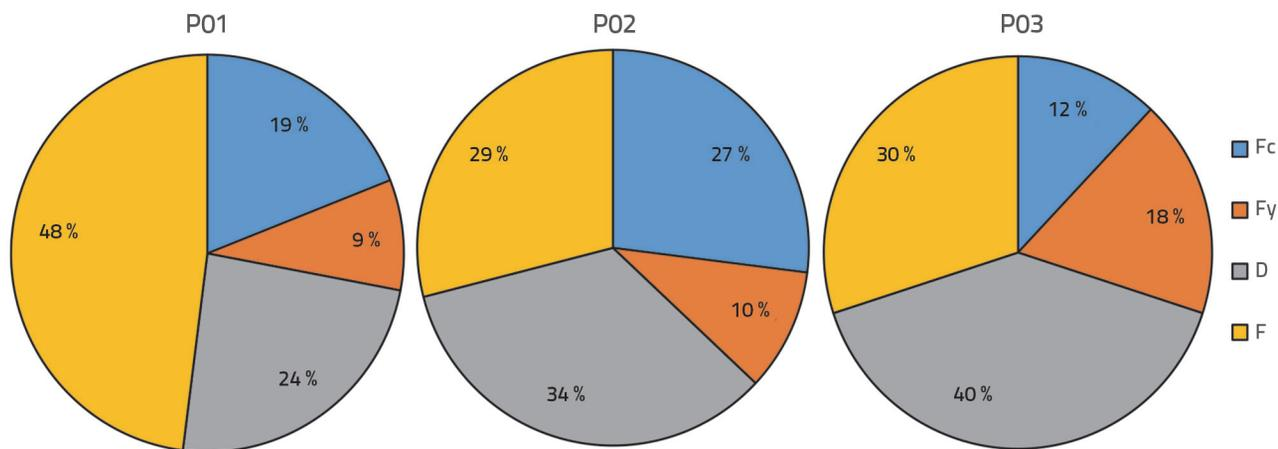
Figure 13. Sensitivity of parameters for single-storey portal
