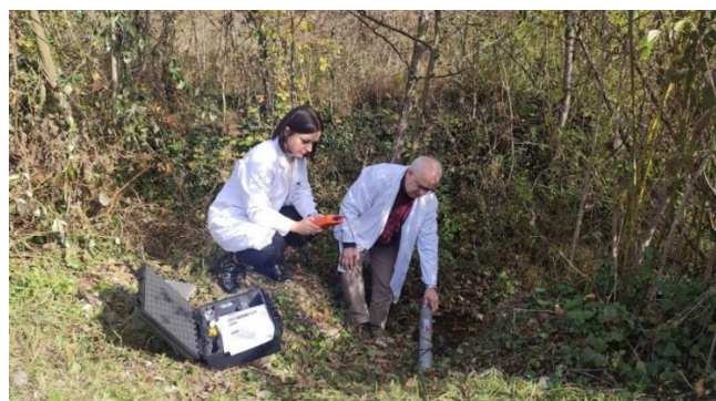
Figure 5: Flow measurement with an Omni TDI 200H ultrasonic meter on site
