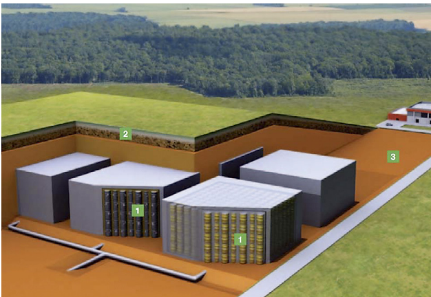
Figure 5: Aube disposal facility disposal concept ( ANDRA, 2011 ) (1) waste package, (2) the final cap, (3) the geological environment of the site (clay aquiclude overlain by a sand aquifer)
