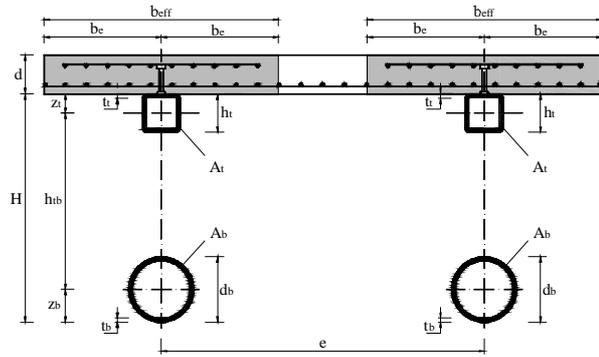
Fig. 2 Vertical cross-section of the composite floor truss system
