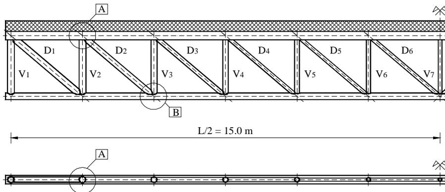
Fig. 5 Arrangement of bracing members
