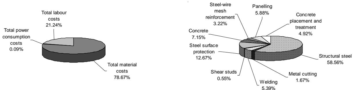
Fig. 7 The distribution of the optimal manufacturing costs of the composite truss system
