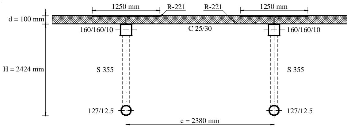
Fig. 4 Optimal cross-section design of the composite floor trusses
