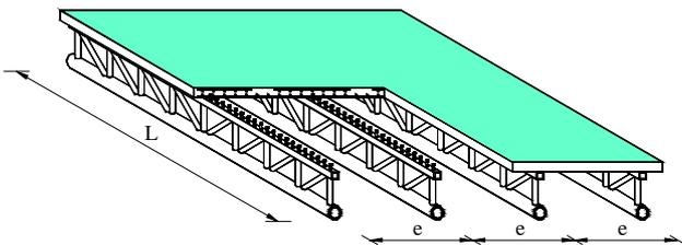
Fig. 1 Composite floor truss system
