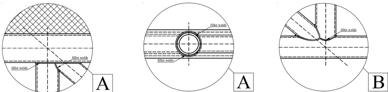
Fig. 6 Design of welded joints
