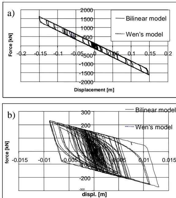
Fig. 4 Comparison of the response obtained by the Wen's and bilinear model: a) for design earthquake; b) for 20% of the design earthquake
