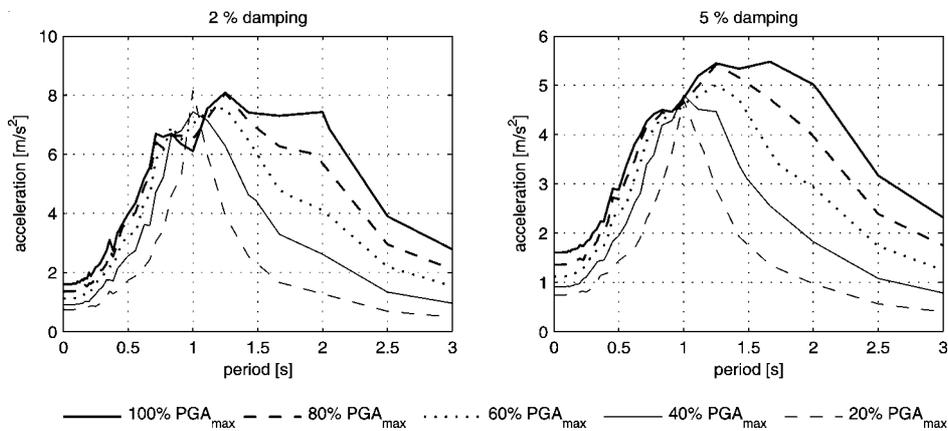
Fig. 8 Floor acceleration spectra in the structure isolated with 3F3D bearings
