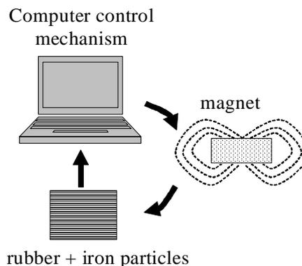
Fig. 10 Scheme of the new isolating MCE device
