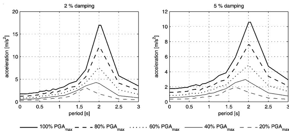
Fig. 9 Floor acceleration spectra in the structure isolated with F3D bearings
