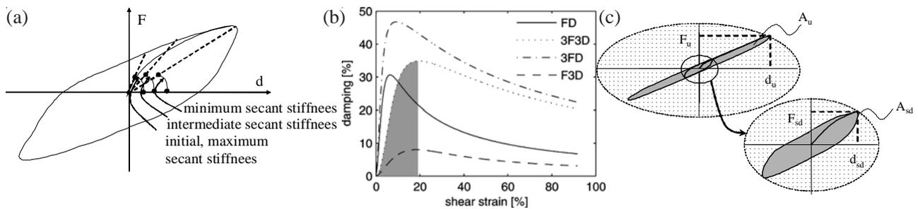
Fig. 7 HDRB: Changes of: a) equivalent stiffness; b) equivalent damping  $\xi_{ef}$ ; and c) calculation of the equivalent damping  $\xi_{ef}$
