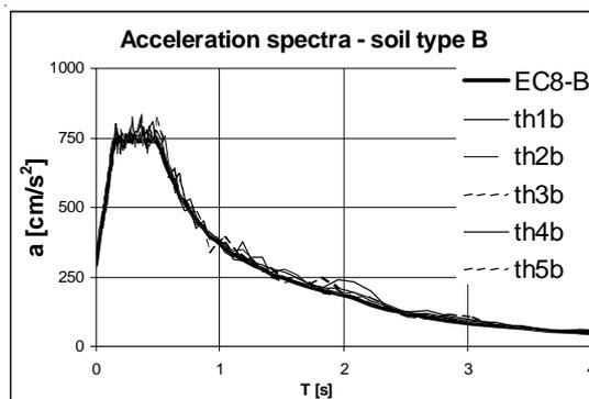
Fig. 6 Spectra corresponding to earthquake input
