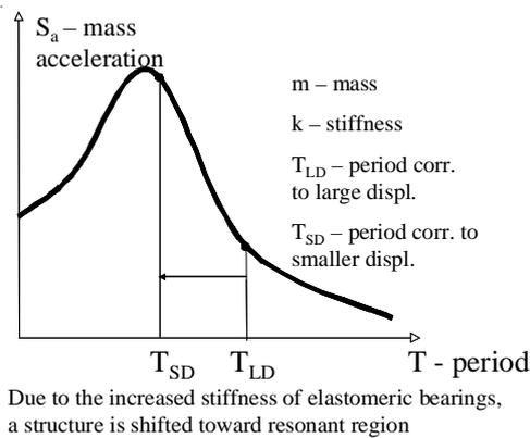
Fig. 1 Due to increased stiffness at weaker earthquakes, the structure is shifted toward the resonant region of the acceleration spectrum
