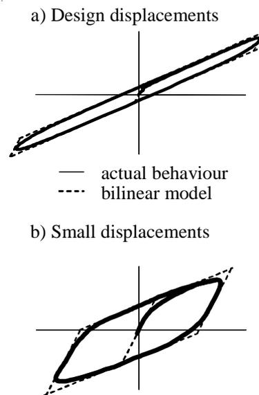
Fig. 2 HDRB: Actual response and response obtained using the traditional bilinear model
