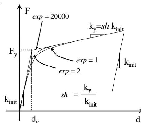
Fig. 3 Wen’s model, used to model HDRB bearings
