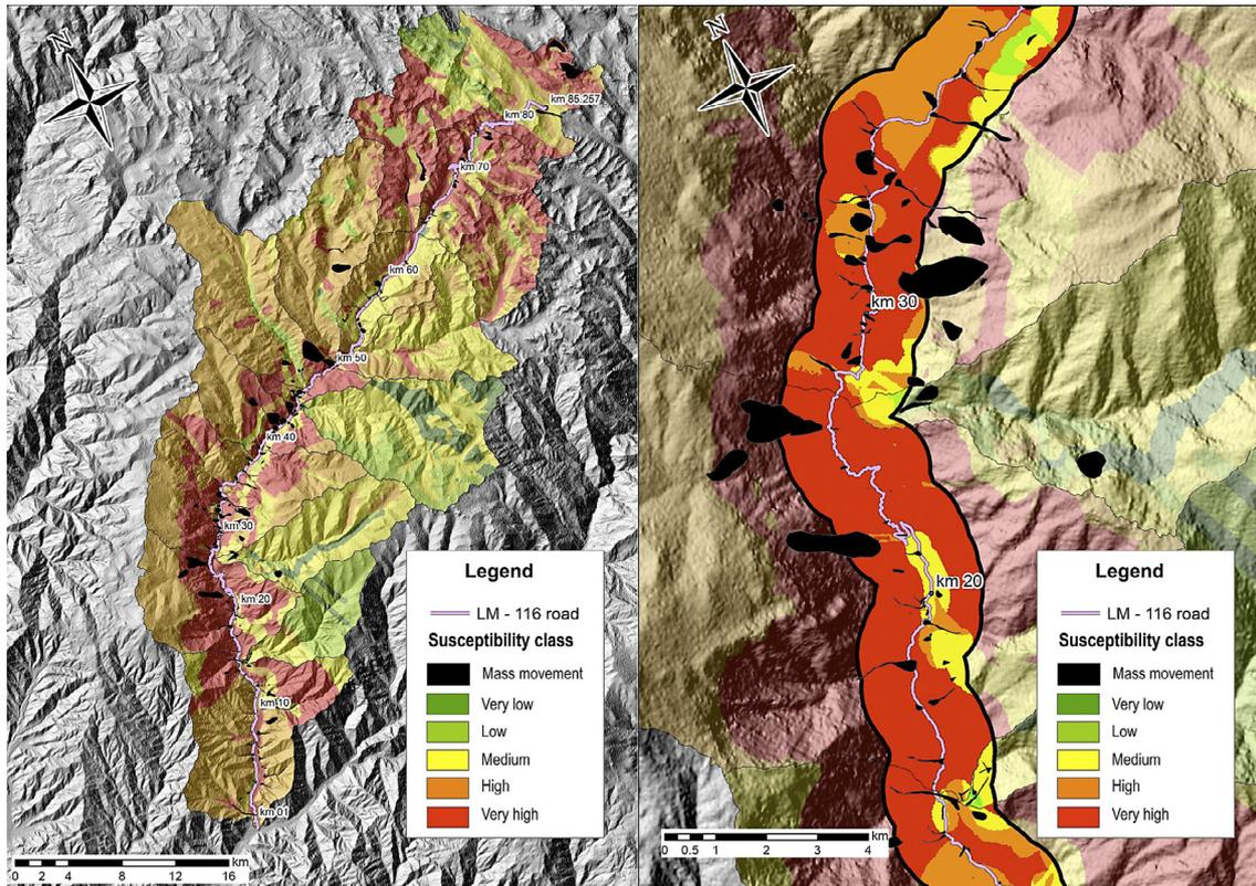
**Figure 7:** Approximation to the mass movements susceptibility Model 4 (Wi methodology). It is observed that the sector located between km 14+000 - km 36+000 presents areas of very high susceptibility.
