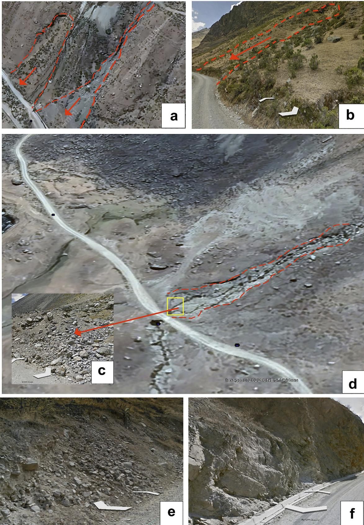
**Figure 3:** Images of some MM occurred in the study area. (a) Translational landslide and debris flow at km 13+250, (b) translational landslide at km 18+250. Figures (c) and (d) show a debris flow affecting the road. Figures (e) and (f) show rockfalls at km 30+000 (Google Earth, 2022).
