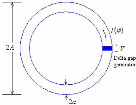
Fig. 1 Circular loop antenna
