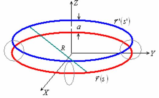
Fig. 2 Circular loop antenna and its associated vectors
