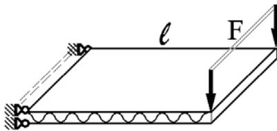
Fig. 5 Simple test case for the metal sandwich optimization problem (width  $b$ )
