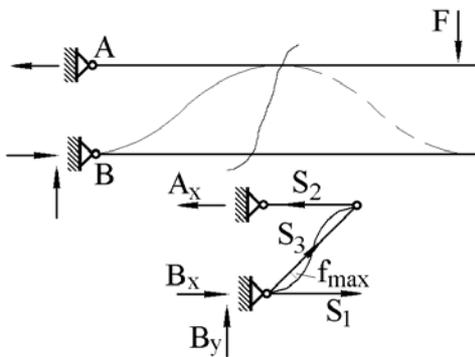
Fig. 4 Simplified model of sandwich plate segment
