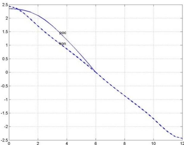
Fig. 9 Optimization of the sandwich plate towards minimum mass of material with constraints on tensile/compressive strength and local buckling of outer plates
