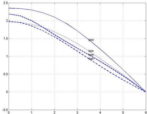
Fig. 13 Change in the constrained optimum shape of the corrugated core for prescribed minimum values of radius of curvature of 3 mm (—), 3.5 mm (-.-) and 4 mm (..) respectively, objective function is the length of corrugated core
