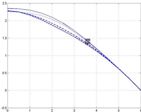
Fig. 12 Change of the constrained optimum shape of the corrugated core for prescribed minimum values of glued bonds of 1.2 mm (—), 1.5 mm (-.-), and 1.8 mm (..) respectively, the objective function is a total cross-sectional area (mass) of aluminum plates
