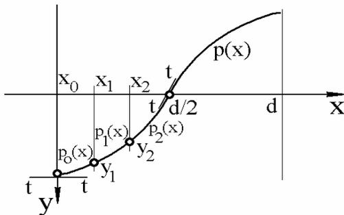
Fig. 3 Piece-wise polynomial interpolation of the shape of corrugated core (basic 3-segment version shown)
