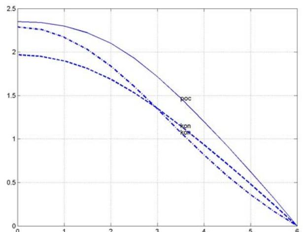
Fig. 11 Optimization of sandwich plate, minimum mass of material (-.-) and minimum length of core (—), all constraints (6)-(12) except technological manufacturability
