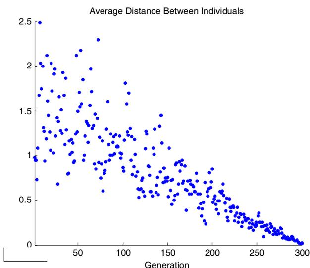
Fig. 15 Convergence of population with the genetic algorithm - based optimization of sandwich plate shown in Figure 14
