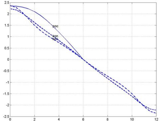
Fig. 10 Optimization of sandwich plate, minimum mass of material (-.-) and minimum length of core (—), constraints on stresses and buckling of both outer plates and corrugated core
