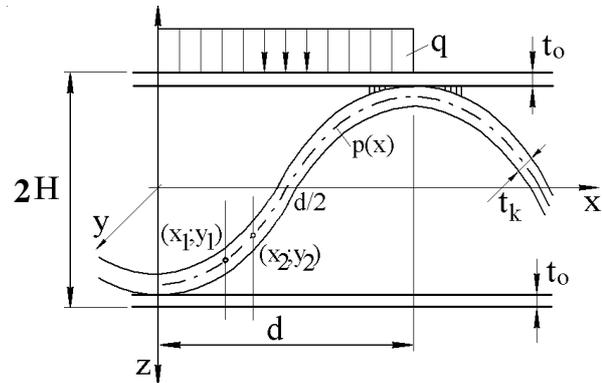
Fig. 2 Geometry of the metal sandwich optimization problem
