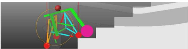
The wheelchair is further up the stairs. The front wheel and the front part of the mechanical system are on the first step, while the rear wheel is still on the ground.                                                                                                                                                         |
