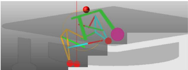
Both the front and rear wheels are now on the second step. The wheelchair is moving up the stairs, and the mechanical system is in a similar configuration to the previous stage.                                                                                                                                              |
