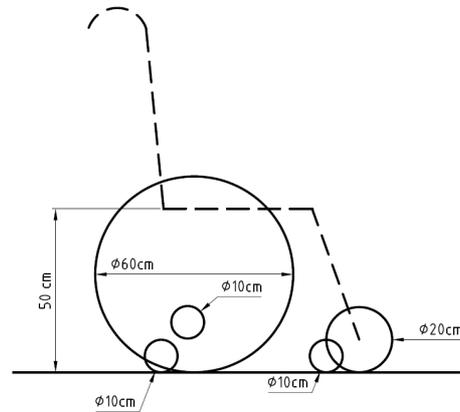
**Fig. 1** Diagram and dimensions of a classic wheelchair
