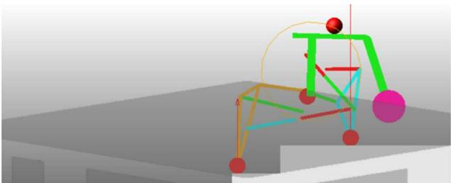
The wheelchair is at the top of the stairs. The front wheel is on the ground, and the rear wheel is on the final step. The mechanical system is stabilizing, and the large front wheel is resting on the ground.                                                                                                               |
