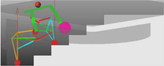
The wheelchair is positioned such that the front wheel is on the second step and the rear wheel is on the first step. The mechanical system is designed to keep the seat area nearly horizontal despite the steep incline.                                                                                                     |
