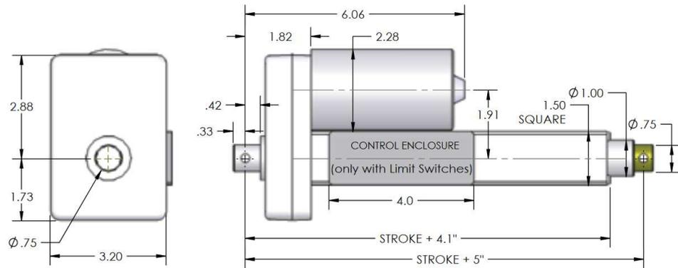
**Fig. 11** Scheme of TMD02 actuator. Dimensions in inches [14]
