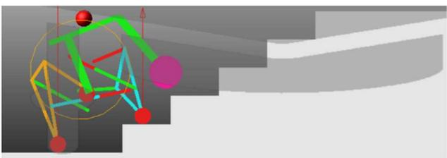
The wheelchair is at a higher point on the stairs. The front wheel is now on the second step, and the rear wheel is on the first step. The entire wheelchair assembly is significantly tilted.                                                                                                                                  |
