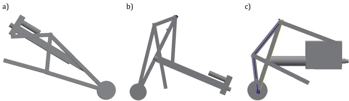
**Fig. 15** Solid model of: a) front mechanism, b) rear mechanism, c) supporting mechanism
