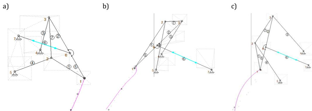
**Fig. 4** Result of the dimensional synthesis: a) for the front mechanism, b) for the rear mechanism, c) for the supporting mechanism
