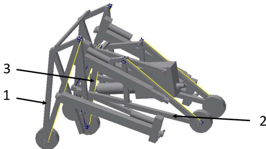
**Fig. 17** View of the mechanisms under the wheelchair, in the folded state; 1 – rear mechanism, 2 – front mechanism, 3 – mechanism of the supporting mechanism
