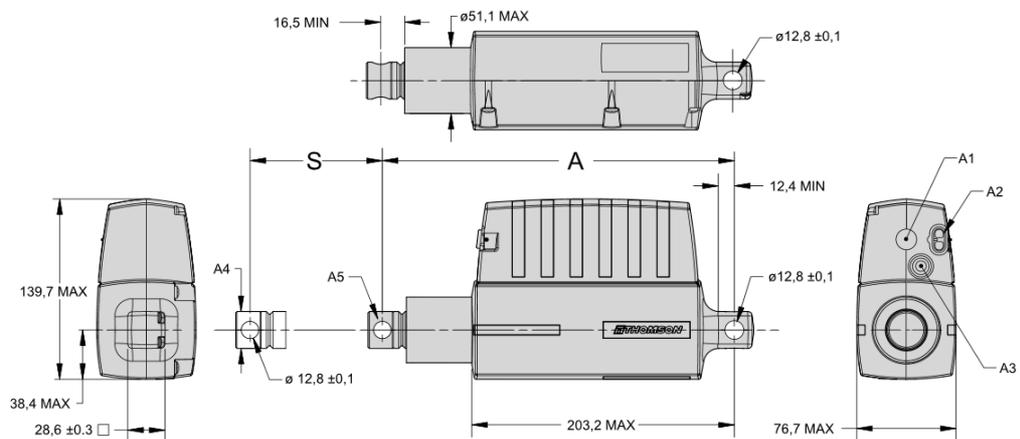
**Fig. 12** Scheme of Electrak Pro actuator [15]
