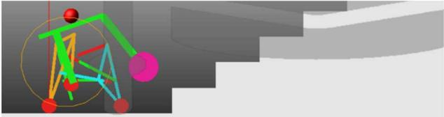
The wheelchair is now on a set of stairs. The front wheel is on the first step, and the rear wheel is on the ground. The mechanical system is tilted upwards to accommodate the incline.                                                                                                                                         |
