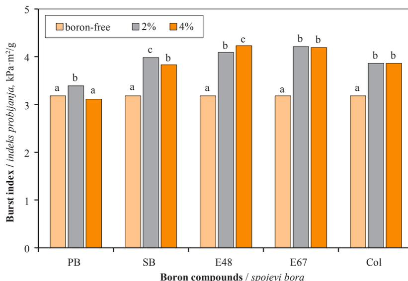
**Figure 4** Effects of boron compounds on burst index of pulps
