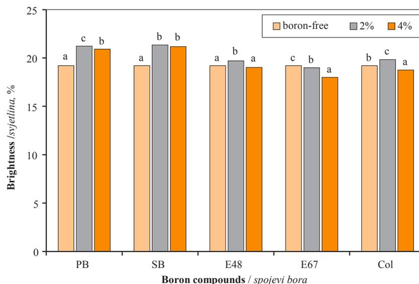
**Figure 6** Effects of boron compounds on brightness of pulps
