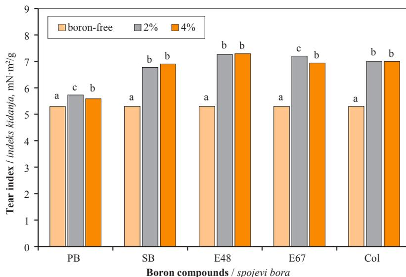
**Figure 5** Effects of boron compounds on tear index of pulps
