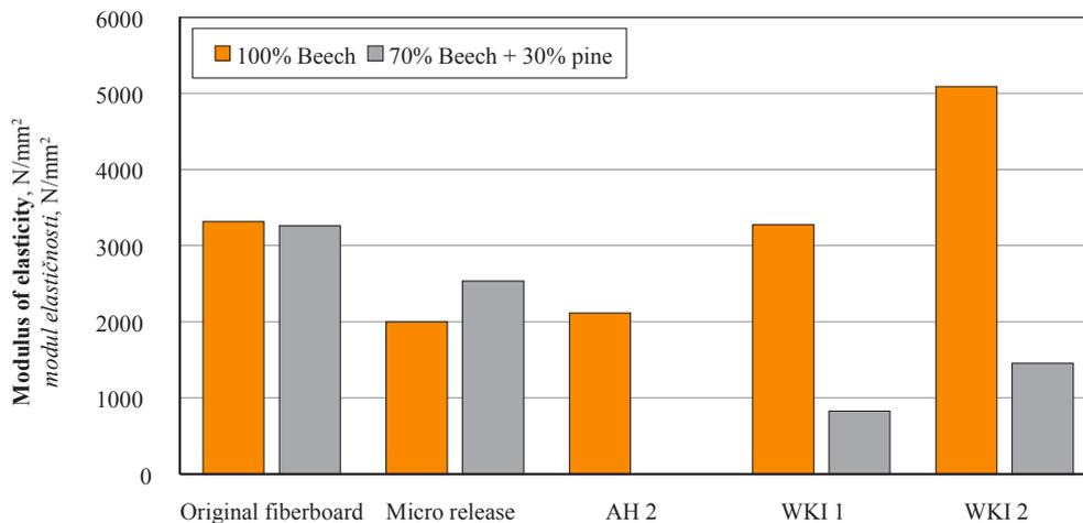
**Figure 4** Modulus of elasticity values of tested boards
