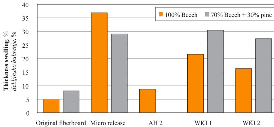
**Figure 2** 24 h thickness swelling values of tested boards
