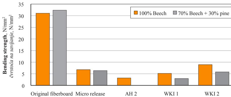
**Figure 3** Bending strength values of tested boards
