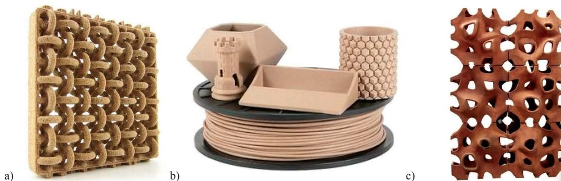
**Figure 2** Examples of printed models: a) SLS technology printed models (<https://3dprint.com/>); b) FDM technology printed model (<https://www.printyourmind3d.ca/products/print-your-mind-3d-woodfill-filament?variant=43074437318>); c) FDM technology printed model (<https://www.forust.com/>)
