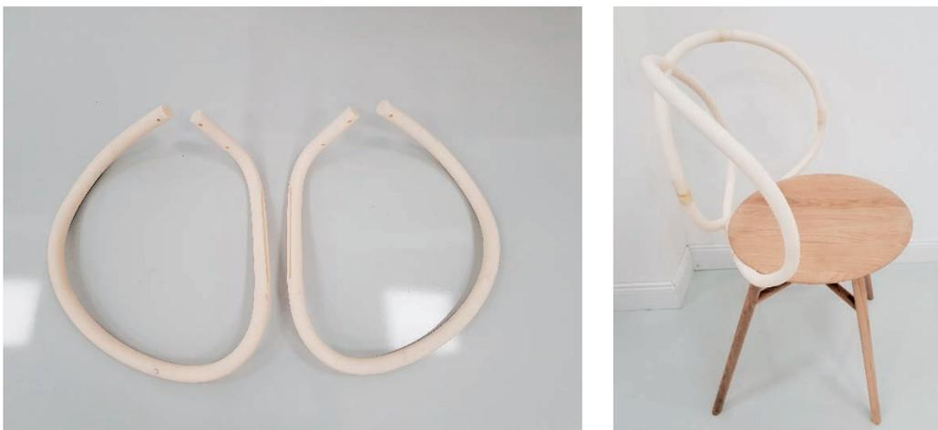
**Figure 6** Example of backrest product development (rapid prototyping) in Croatian furniture manufacturing; (Jarža, L., photography, 2022)
