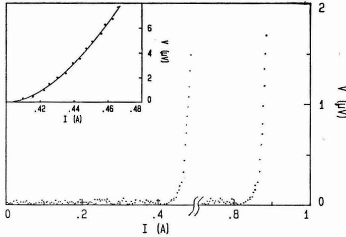
Fig. 7. Initial parts of  $V$ - $I$  curves for an YBaCuO sample at two different temperatures (80 K and 70 K, respectively). The inset: A fit of the experimental points to the power law  $V(I) \simeq (I - I_c)^n$ .
