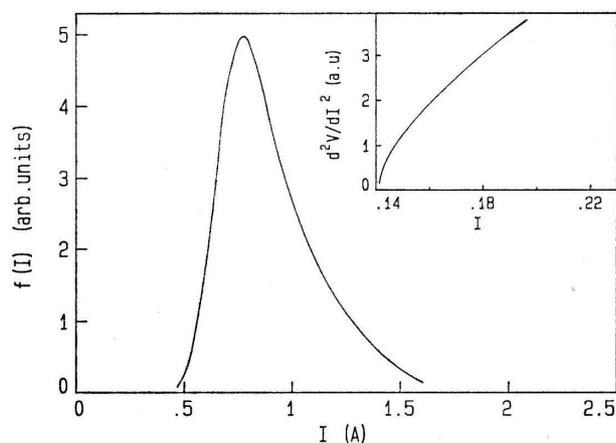
Fig. 8. Critical current distribution (CCD) for YBaCuO sample from Fig. 7 at 80 K. The inset: initial part of CCD curve for the sample at 85 K shown in an expanded scale.
