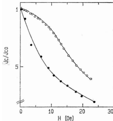
Fig. 4. Variation of critical current at 80 K (normalized to its value in zero applied field) with magnetic field (1 Oe = 79.5 A/m) for two ceramic YBaCuO samples exhibiting self-field limited ( $\circ$ ) and intrinsic ( $\bullet$ ) behaviour, respectively.
