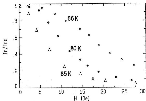
Fig. 6. Variation of normalized critical current with magnetic field (1 Oe = 79.5 A/m) for an YBaCuO sample exhibiting the self-field limited behaviour at different temperatures.
