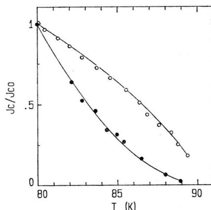
Fig. 5. Variation of normalized critical current with temperature for two ceramic YBaCuO samples exhibiting self-field limited (o) and intrinsic (•) behaviour, respectively.
