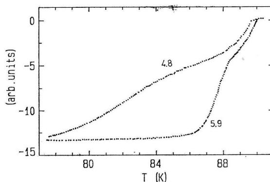
Fig. 3. AC susceptibility of YBaCuO samples with different densities (4.8 and 5.9  $\text{g cm}^{-3}$ , respectively) as a function of temperature.
