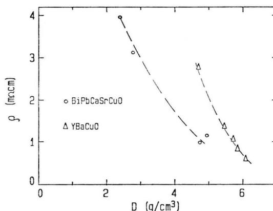
Fig. 2. Variation of resistivity at 300 K with density for ceramic YBaCuO ( $\Delta$ ) and BiPbSrCaCuO ( $\circ$ ) samples.
