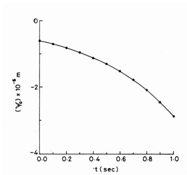
Fig. 2. The response of a piezoquartz bar under input signal varying exponentially with time and acting for a finite interval.
