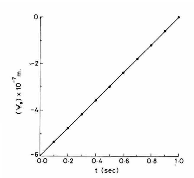
Fig. 1. The response of a piezoquartz bar under input signal varying linearly with time and acting for a finite interval.
