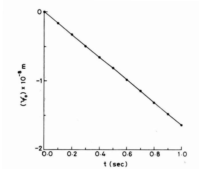
Fig. 3. The response of a piezoquartz bar under input signal varying periodically with time and acting for a finite interval.
