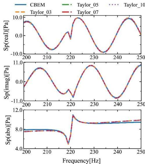
**Fig. 12** Comparison of sound pressure between the BEM based on Taylor expansion and the traditional BEM at frequency range [200,250] Hz
