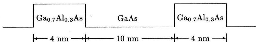
Fig. 1.  $\text{Ga}_{0.7}\text{Al}_{0.3}\text{As}$ -GaAs- $\text{Ga}_{0.7}\text{Al}_{0.3}\text{As}$  quantum well.
