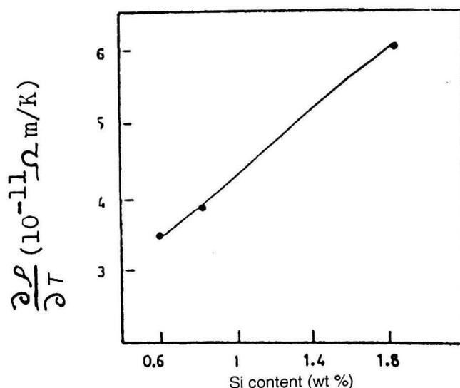
Fig. 3. Dependence of  $(\partial\rho/\partial T)$  on silicon content.
