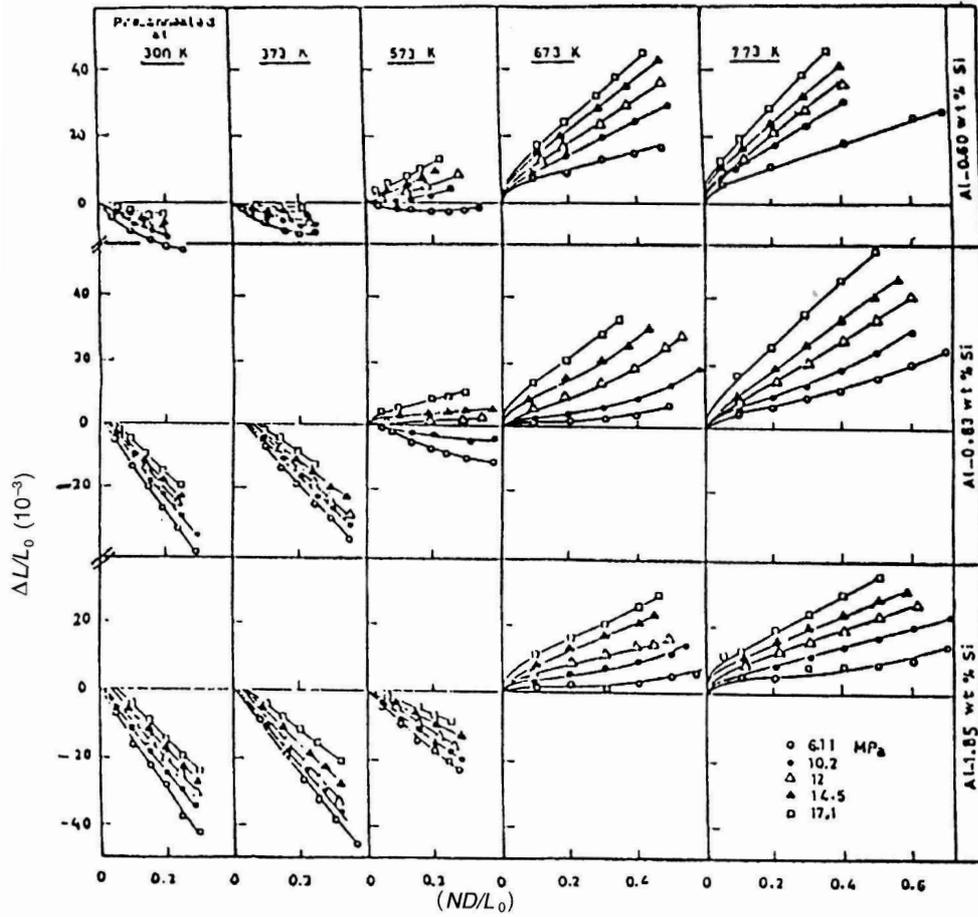
Fig. 1. Room temperature variation of tensile strain  $\Delta L/L_0$ , due to torsional deformation  $ND/L_0$  for samples of the three (Al-Si) alloys, untreated (300 K) and pre-annealed at temperature of 373, 573, 673 and 773 K, and strained by axial tensile stresses of 6.11, 10.2, 12, 14.5 and 17.1 MPa.
