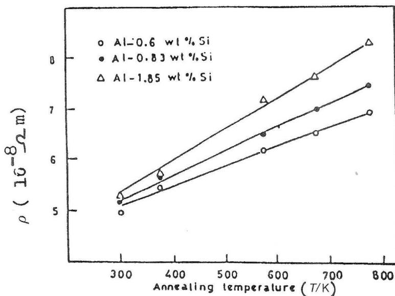
Fig. 2. Dependence of resistivity of samples on pre-annealing temperature for the three alloys.
