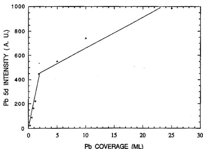
Fig. 1 Evolution of the intensity of Pb 5d core level line during the deposition of Pb onto the Si(111)1 × 1-H surface.
