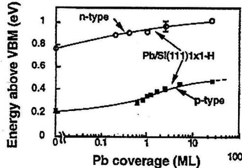
Fig. 4 Surface  $E_F$  position as a function of Pb deposition. The position for Si(111)1 × 1-H corresponds to the flat band conditions.
