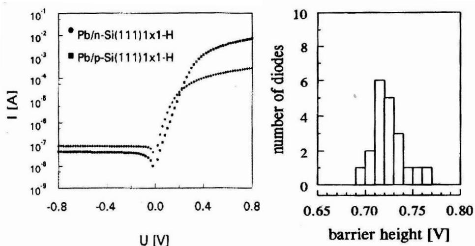
Fig. 2. Typical  $I - V$  curves of Pb/n-Si(111)1 × 1-H and Pb/p-Si(111)1 × 1-H diodes. The contact area was  $6.4 \times 10^{-7} \text{ m}^2$ .
