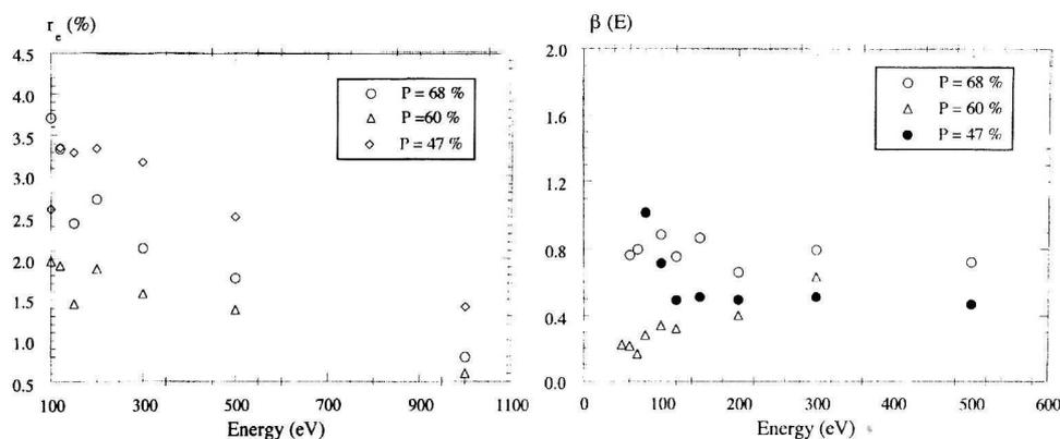
Fig. 1. Variation of elastic reflection coefficient,  $r_e(E)$ , with the porosity  $P$ .
