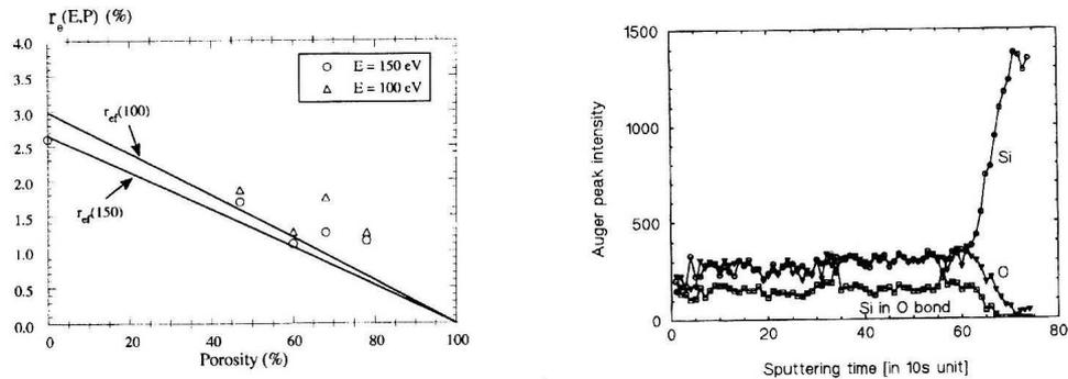
Fig. 3. Elastic reflection coefficients,  $r_e(E)$ , for  $E = 100$  and  $150$  eV, plotted versus porosity ( $P$ ). They are above the “fictive” straight lines characterizing elastic reflection of the intact Si surface area, not covered by voids.  $r_{ef}(E) = (1 - P/100)r_{eSi}(E)$ .  $r_{eSi}(E)$  was measured with a HF treated Si wafer.
