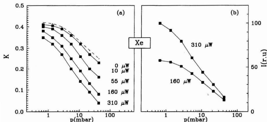
Fig. 4. (a) Plot of the optical depths  $K = k_{791.3}^0 L$  of the barium 791.3 nm line vs. xenon pressure in dependence on the laser beam power. The dashed line represents the extrapolation to zero power (1 bar =  $10^5$  Pa). (b) The relative fluorescence intensity of the barium 791.3 nm line as a function of the xenon pressure, obtained for the two different pumping powers.
