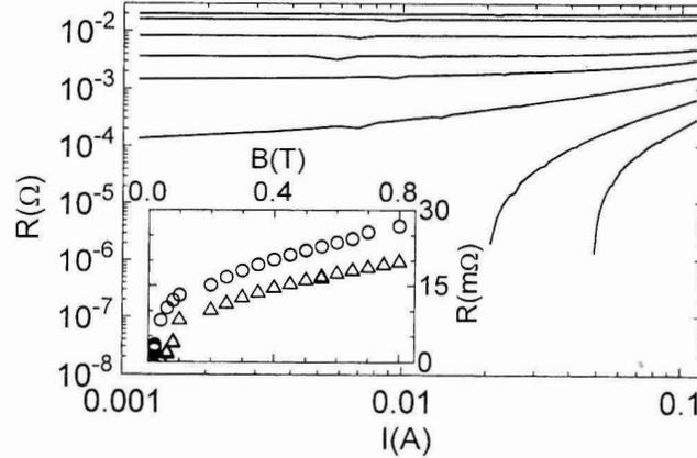
Fig. 5. Plot of resistance vs. current for the bare core of Ag-Bi 2223 tape at  $T = 100$  K for fields  $B$  (parallel to  $c$ -axis) = 0.01, 0.02, 0.04, 0.06, 0.08, 0.1, 0.5 and 0.8 T (bottom to top). The inset: plot of the Ohmic resistance vs. field  $B$  for a bare core of the Bi 2223 tape at  $T = 100$  K ( $\Delta$ ) and 103 K ( $\circ$ ). Note the flux-flow at higher  $B$ .
