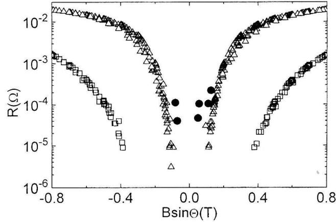
Fig. 3. Plot of resistance versus magnetic field component  $B \sin \Theta$  (perpendicular to the plane of the tape) for the sample described in Fig. 2, at temperatures  $T = 85$  K ( $\square$ ) and 95 K ( $\triangle$ ). ( $\bullet$ ) denotes data for  $\Theta \leq 10$  at 95 K.
