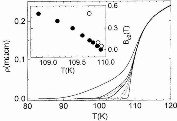
Fig. 2. Resistive transitions for the core of Ag-Bi 2223 tape in field:  $B = 0, 0.05, 0.1$  and  $0.5$  T (right to left) applied parallel (---) and perpendicular (—) to the plane of the tape. The inset: the plot of upper critical fields  $B_{C2}^c$  (●) and  $B_{C2}^{ab}$  (○) for the same tape versus temperature.
