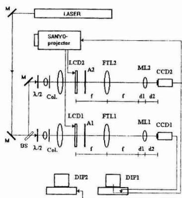
Fig. 1. Scheme of the experimental setup; M: mirror; BS: beam splitter; Col.: collimator; LCD1, LCD2: liquid crystal displays; A1, A2: polarizers; FTL1, FTL2: Fourier transform lenses; ML1, ML2: magnification lenses; DIP1, DIP2: digital image processing systems.
