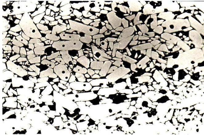
*Fig. 2. Microstructure of sample 1, sintered 4 hours at 1700 °C, magnification: ×270.*
