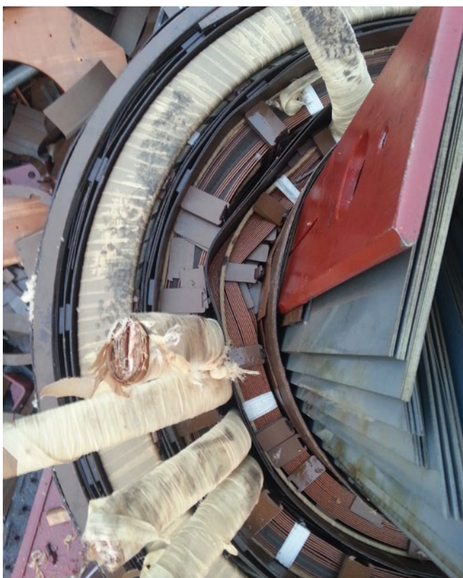
Figure 3.2. Forced buckling of LV winding
