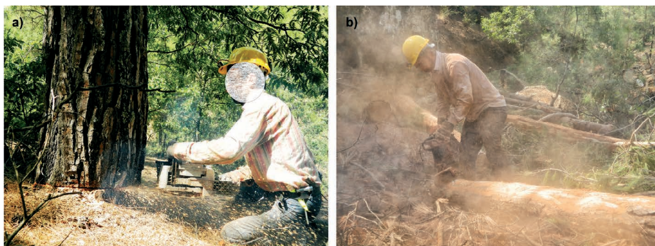
Figure 3. The moment of exposure to emitted exhaust gases from the chainsaw for an operator using low-standard work safety equipment (a: tree felling with chainsaw, b: debarking with chainsaw)
