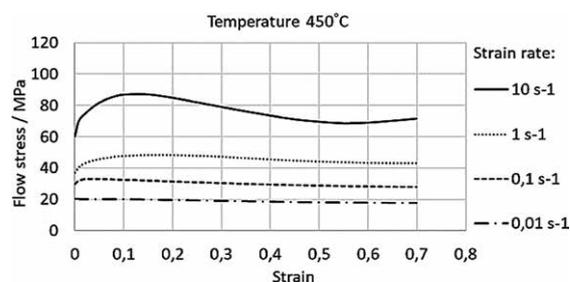
**Figure 6** Flow stress curves of ZK60 cast alloy at a temperature of 450 °C
