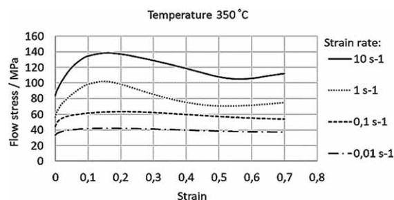
**Figure 4** Flow stress curves of ZK60 cast alloy at a temperature of 350 °C
