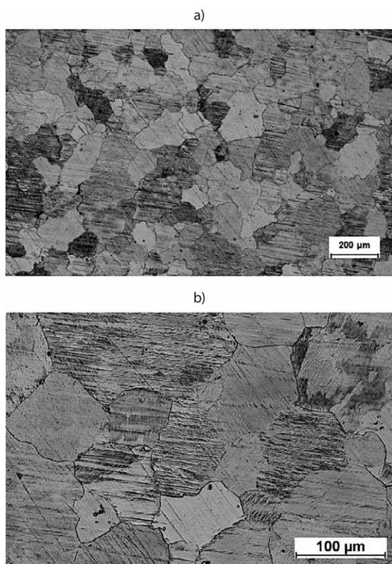
**Figure 3** Microstructures of homogenised ZK60 cast magnesium alloy with magnification 50 x (a) and 200 x (b)
