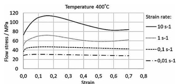
**Figure 5** Flow stress curves of ZK60 cast alloy at a temperature of 400 °C
