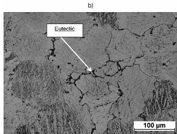
**Figure 2** Microstructures of as-cast ZK60 magnesium alloy with magnification 50 x (a) and 200 x (b)
