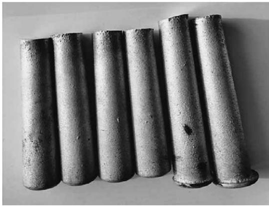
**Figure 1** Ingots cast from ZK60 magnesium alloy
