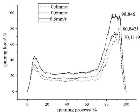
**Figure 8** Relation diagram of spinning pressure and feed ratio
