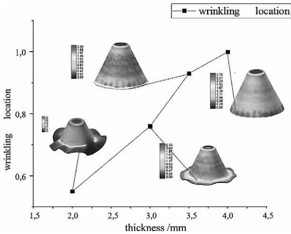
Figure 5 Wrinkle of different wall thickness
