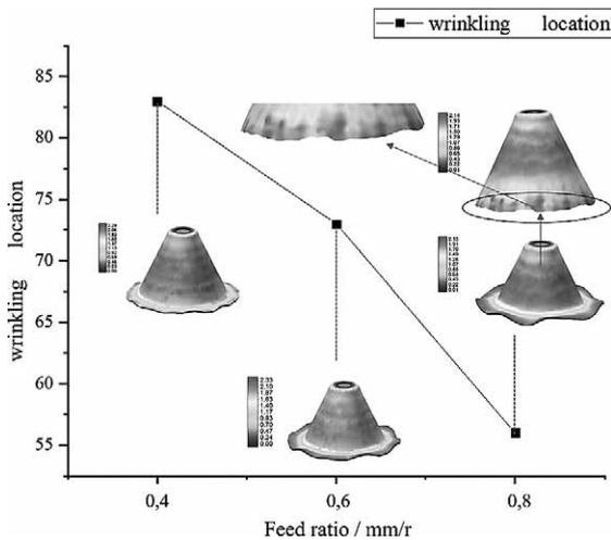
Figure 6 Wrinkles with different feed ratios
