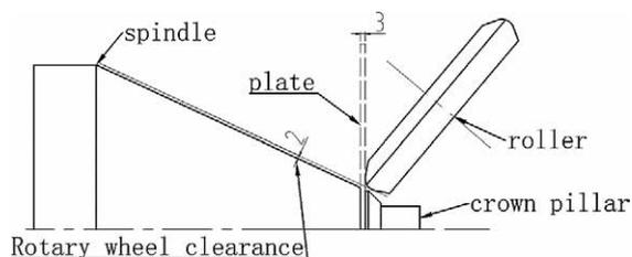
Figure 1 Power spinning schematic diagram
