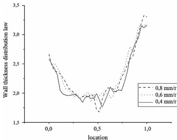
Figure 4 Effect of feed ratio on wall thickness
