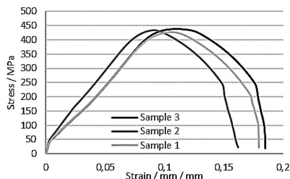
**Figure 7** Stress-strain curve for selected samples after cold working
