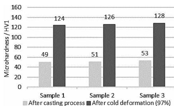
**Figure 6** Measurement results of Vickers microhardness in the cross-section of samples after casting process and cold working
