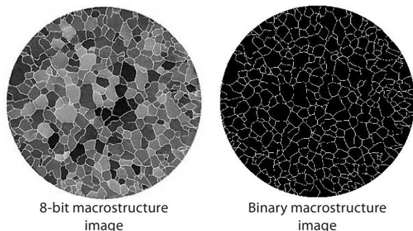
Figure 1 Converting an 8-bit image macrostructure to binary in ImageJ software
