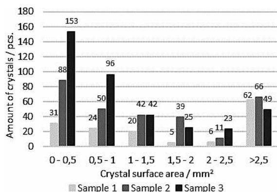
**Figure 5** Measurement results of the mean size of crystals in the cross-section
