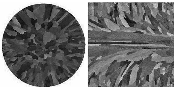
**Figure 4** Macrostructure of sample 3 – casting speed 0,22 m / min
