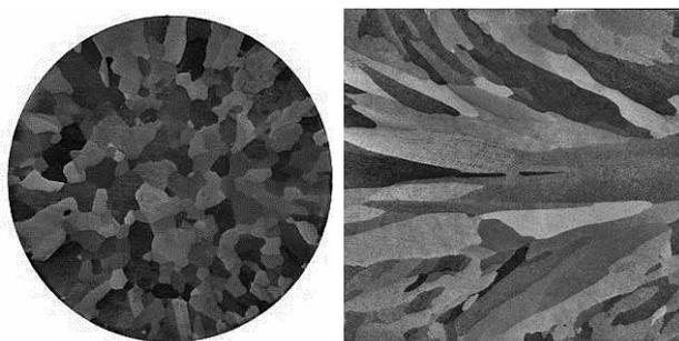
**Figure 3** Macrostructure of sample 2 – casting speed 0,13 m / min
