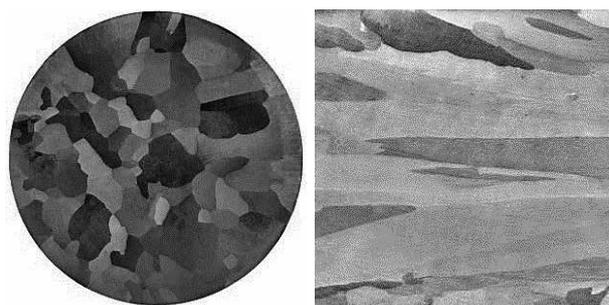
Figure 2 Macrostructure of sample 1 – casting speed 0,09 m / min
